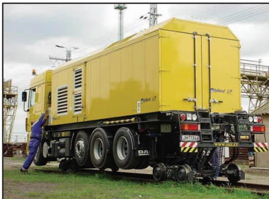
While Robinson Custom Enclosures is best known for its enclosures for stationary engine systems primarily used in power generation, the company's capabilities extend well beyond a single industry. A good example was a highly specialized enclosure for a mobile track welding machine. The enclosure had to fit within very tight dimensional and weight specifications in order to be able to operate in small European rail tunnels.
