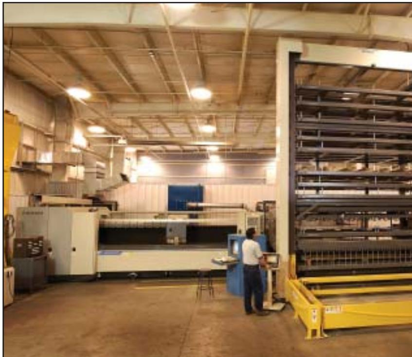
Robinson recently purchased two Mitsubishi 5000W CNC laser cutting tools. These machines include in-line towers that automatically feed all of the materials for the cutting processes. The machines' automation and accuracy increases quality and reduces physical handling of the materials.
