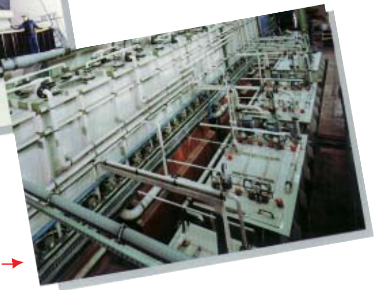
Autoclave pickling line for stainless steel tubes
