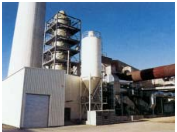
DESO x scrubber downstream of a rotary kiln with gypsum as end product
